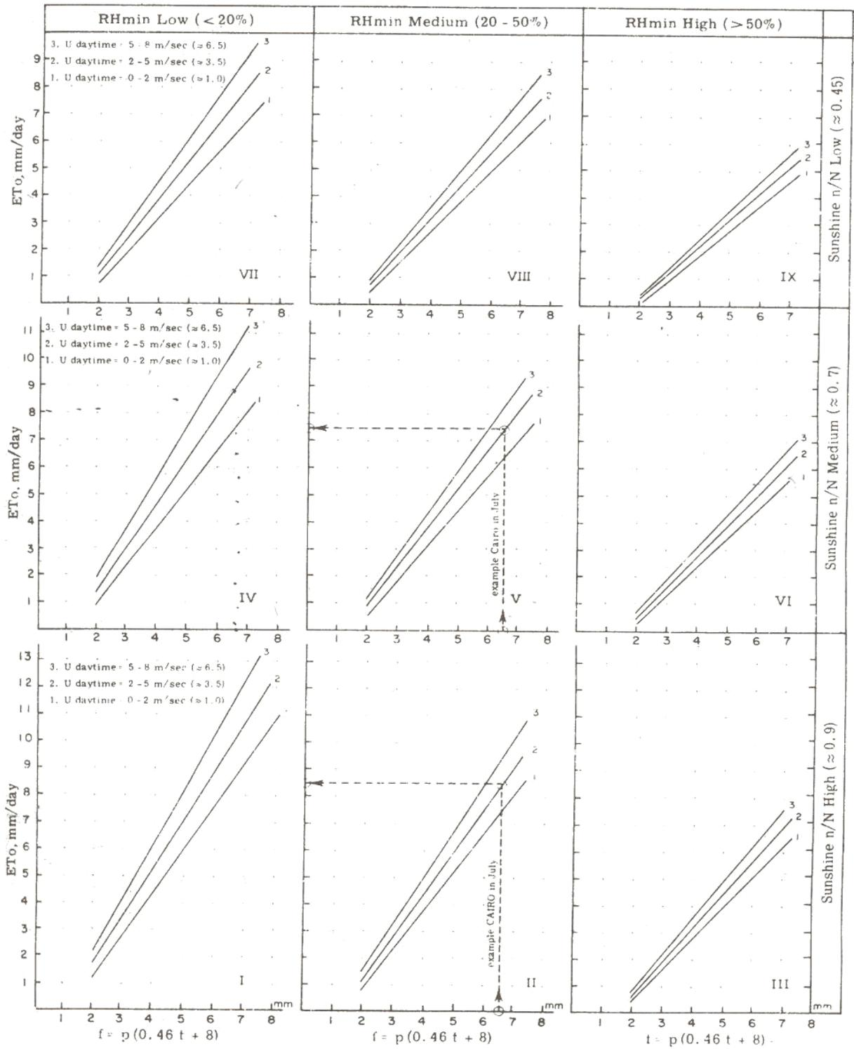
Figure - 1: Prediction of ET<sub>0</sub> from Blaney-Criddle f-factor for different conditions of minimum relative humidity, sunshine duration and day-time wind
