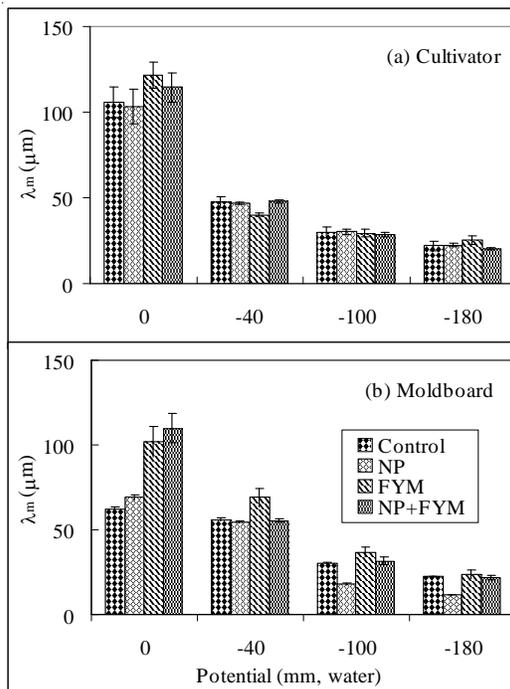
Figure - 4: Characteristics mean pore radii (Ankeny, 1992) as affected by the long-term treatments. Treatments and the bar as defined in the caption of Figure 1.
