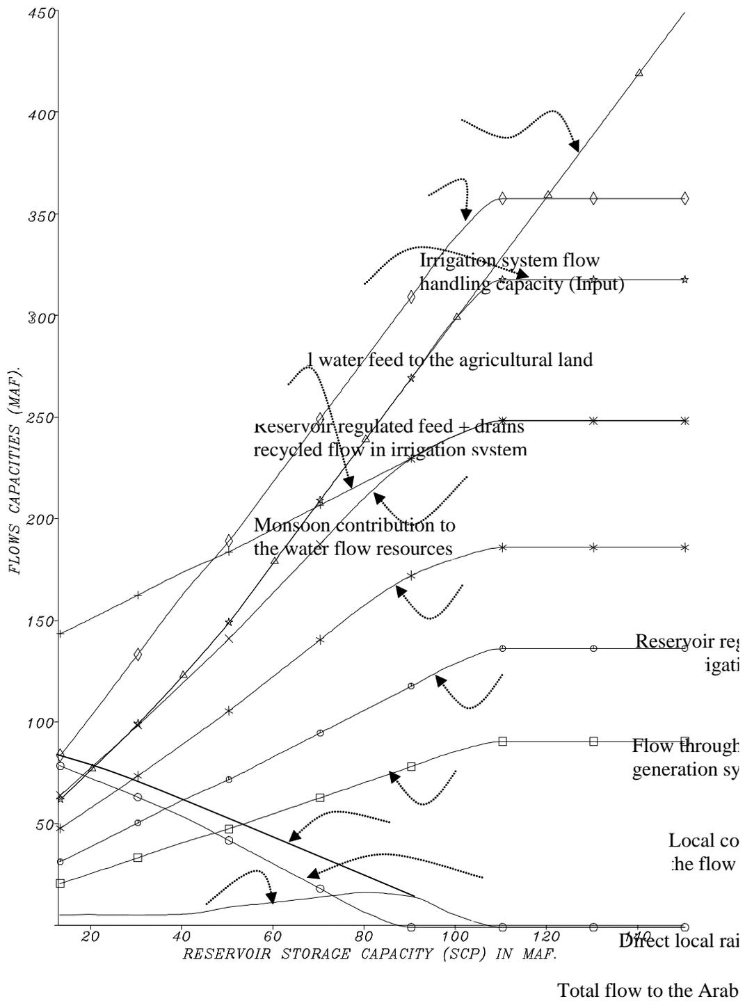
**Figure - 5: Reservoirs Capacity Effect on Related Flow Quantities**
